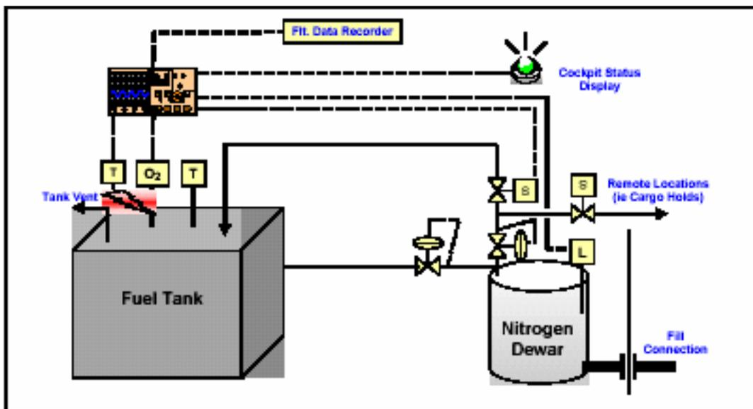
*Liquid nitrogen has a purity of 99.997%, therefore the amount of nitrogen required for inerting is reduced substantially. The OBIGGS systems discussed in the FTIHWG report generate nitrogen with a purity of 95%. The volume of nitrogen required using lower purity nitrogen is about 75% higher than would be required for liquid nitrogen. It is argued that the cost of inerting with higher purity nitrogen is lower than for lower purity (see "The Effect of Nitrogen Purity on Ullage Washing" below).*
