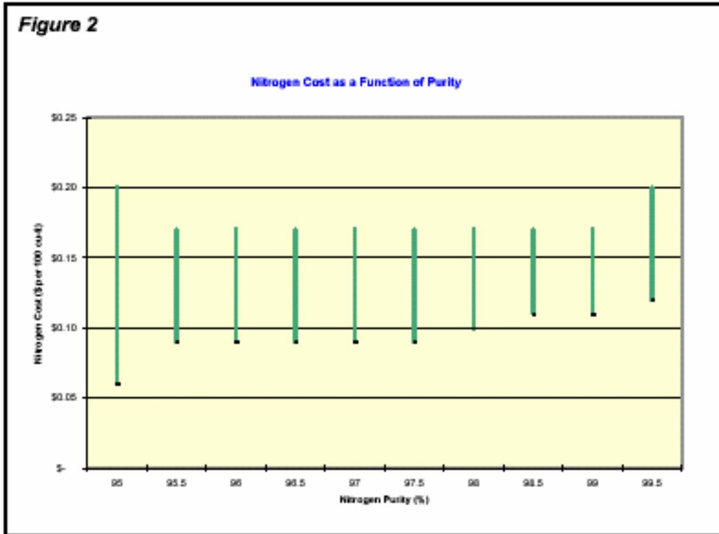
**Figure 2 Nitrogen Cost as a Function of Purity**
